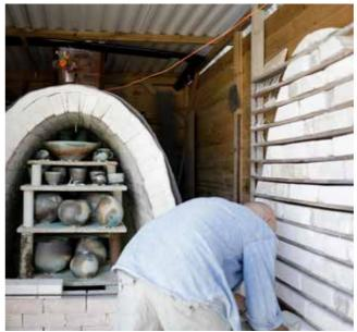
**16** The wicket is taken down and the bricks put in their place until next time. I'm happy with what I can see so far – the temperature looks to have been even throughout the kiln and the colours and surfaces have developed well. It's time to get the pots unpacked and start them on the next part of their journey to a gallery or new owner.
