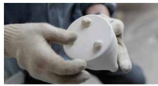
**2** The wadding is mixed with just enough water to make a firm but pliable material. Each piece will need at least three pieces to support it through the firing. Any left over wadding is rolled into a thin slab then cut into disc shapes with a pastry cutter. These are dried and can be used in the next firing.
