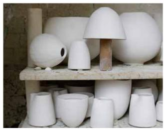
**3** Sometimes I pack pieces upside down or on their side. This means that the soda vapour will touch them in different directions producing a variety of flashing marks. Here the small round pod form (left) is placed on three sea shells, which will prevent it from sticking to the shelf.
