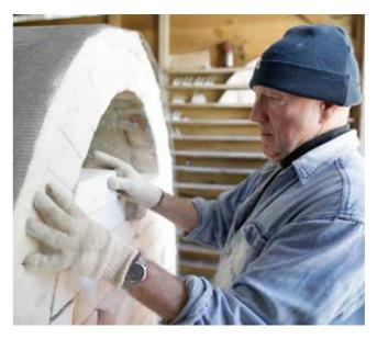
**7** Once the kiln is full, the wicket is carefully bricked up, building in spraying ports between each layer of shelves. There are usually eight or nine of these. The cones also need to have their own spy hole. The door bricks are stored on shelves close to the kiln.
