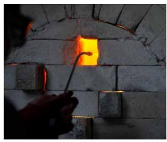
**12** I have a stainless steel sprayer that allows me to spray the sodium mixture deep into the kiln. I spray for about ten seconds into each port, moving quickly from one to the next. The process including mixing takes about one hour.
