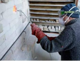
**10** After a slow start, the firing proceeds in a conventional way until cone o6 bends. I then start a reduction/ oxidation sequence. I use a combination of slide and passive dampers to change the atmosphere in the kiln. I gauge the changes in atmosphere by looking at the length of the flame that emerges from the spy holes.
