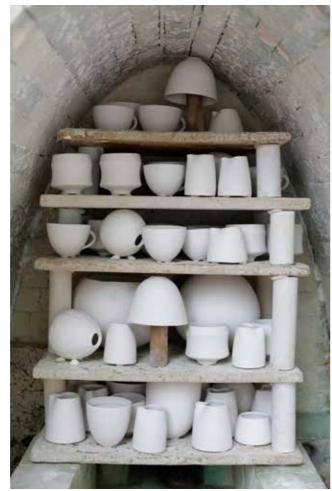
**4** The back section of the kiln is nearly completed. I try to leave spaces for the sodium vapour to reach through all of the chamber. I use wadding to separate the shelves and props. All of the pieces have been given a covering of porcelain slip containing 2% copper carbonate. This is applied when the pots are dry. They are dried again before firing. At this point everything is an off- white colour.
