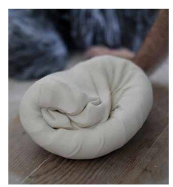
1 Porcelain is not difficult to use, providing you remember that its physical properties are different from any other type of clay. I've used the same porcelain clay for many years – 1149 HF porcelain from Potclays. I mix the new clay with an equal quantity of reclaim in a de-airing pugmill. I like to mix and store the clay for as long as possible, it is then wedged and kneaded to remove the air before use.
