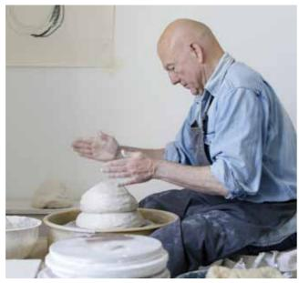
4 The second and any subsequent pieces are added and joined using a rhythmic beating action with both hands slapping inwards and downwards. This begins to amalgamate the clay into a homogenous lump and is done while the wheel is rotating slowly.
