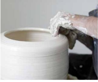
17 The wide rim is started by thinning the top section of the form and then bending this almost horizontally. It's a tricky operation as the clay is now very soft. Any clumsy pressure or movement will make the thinned edge collapse. Throughout this stage I support the rim with gentle finger pressure underneath.
