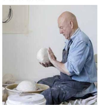
3 When I add the next piece, I take care not to trap any air. I smooth the surfaces that will be joined with my fingers and squeeze the clay to form two convex shapes.
