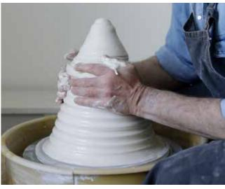
6 For me, coning the clay is an important stage in throwing porcelain. It helps to remove any remaining unevenness left after joining the pieces and compresses the clay, which helps to prevent cracks forming during drying and firing.
