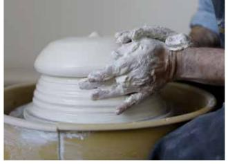
8 As I re-centre the clay it forms a mushroom shape. At this early stage I use my right hand on the top to press downwards and my left on the outside to stop the clay from folding over and trapping air.
