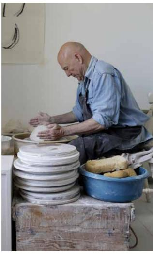
**2** For my larger forms the clay is prepared in amounts weighing roughly Tokgs. This is a comfortable quantity to knead thoroughly by hand and I often use these pieces in multiples. The first piece of clay is placed on a dampened wheel head and slapped firmly into place.
